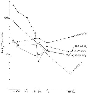
FIG. 8. Chrondrite-normalized REE patterns for five representative rocks covering the range of basic, intermediate, and acidic compositions from the Kemiö-Orijärvi-Lohja belt.
